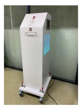
Input power: Wavelength: Type of ultraviolet lamp: Dimensions\*: Air exchange rate (ACH): Input voltage: Ambient noise: Total UV irradiation intensity: 300 watts 253.7nm induction UV light 15.8" L x 13.8" W x 59.3" H 200-1000 CFM (tunable) 120-277 volt, 47Hz – 60Hz 50 db 1335 uW/cm2
