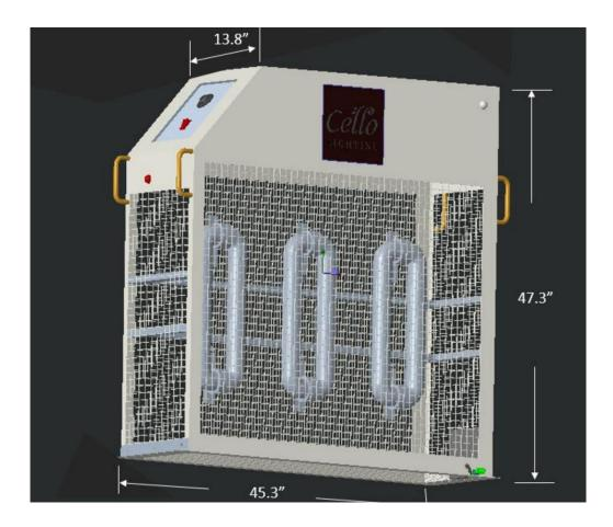
Input power: Wavelength: Type of ultraviolet lamp: Dimensions\*: Air exchange rate (ACH): Input voltage: Ambient noise: Total UV irradiation intensity: 1000 watts 253.7nm induction UV light 45.3" L x 13.8" W x 59.3" H (assembled) 200-2000 CFM (tunable) 120-277 volt, 47Hz – 60Hz 50 db 4005 uW/cm2
